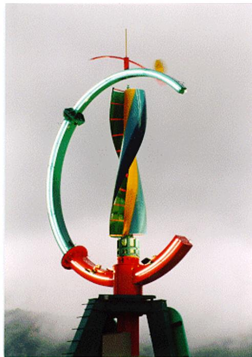
*A typical Savonius type turbine*
