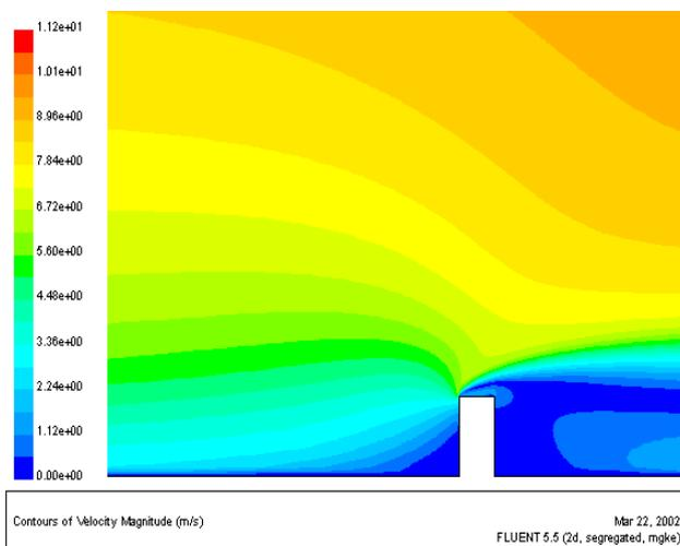
This figure makes it apparent that wind passes at an upward angle of 30 to 40 ° from the leading edge over the roof of the building. Underneath that line there is only turbulence and no wind. For that reason the turbine must be placed on a mast of sufficient height to bring it turbine above the turbulence.
