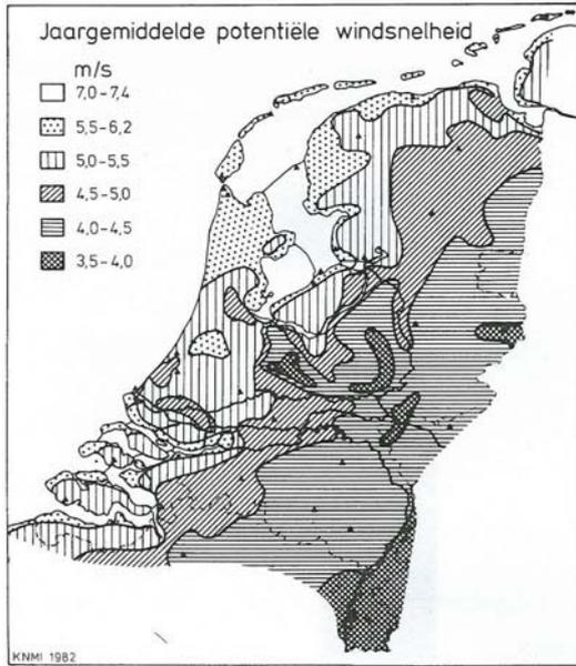
In cooperation with the Institute for Wind Energy of the Delft University of Technology the Turby team has developed a program to calculate the wind speed distribution at different heights and terrain roughnesses and used that to calculate the yield for one hundred areas in the Netherlands (distinguished by the first two numbers of the postcode) based on these data.
