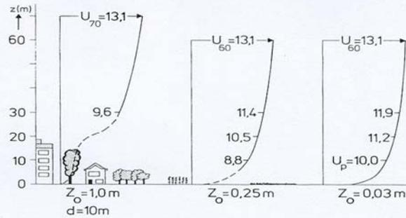
*Windspeed profiles above different terrain roughness  $z_o$  (and displacement height  $d$ ) at a mesoscale wind speed
