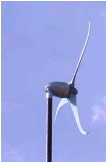
Figure 10. Swept blades were tested with a prototype nacelle on a free standing tubular tower.
