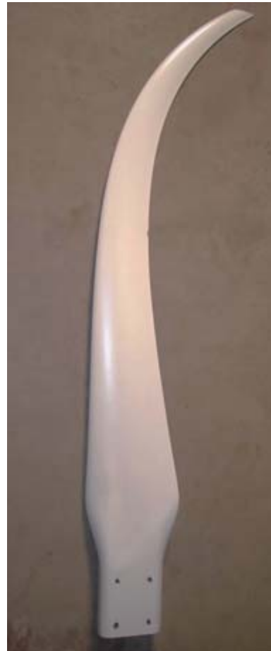
Figure 11. Southwest believes swept blades have promise for reducing aeroacoustic noise. These prototype blades will be tested at the NWTC.
