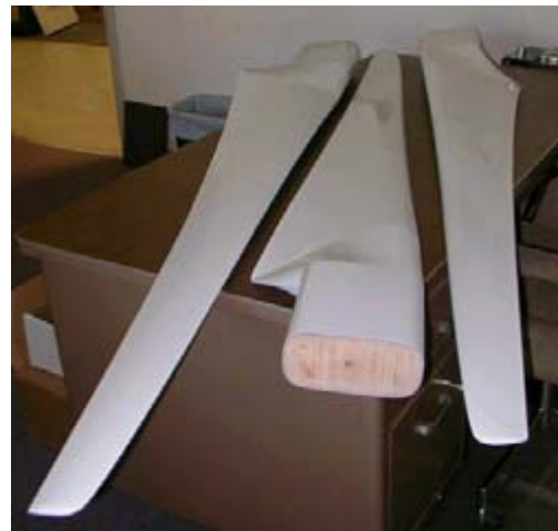
Figure 8. Pre-prototype blade set for 1.8 kW turbine tested by Southwest in Flagstaff, Arizona.
