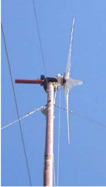
Figure 9. This pre-prototype test turbine, shown with straight blades, was used to investigate various configurations.
